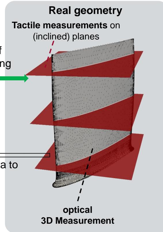
Definition and analysis of sections according to drawing
